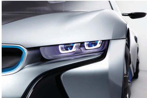
BMW is promising laser-diode-based headlights for the production version of its i8 concept car.
